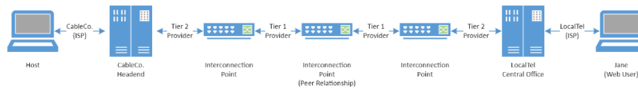
Figure 1. A graphical representation of the point-to-point vision of the internet. Adapted from Tejas N. Narechania & Erik Stallman, Internet Federalism, 34 HARV. J.L. & TECH. 547 (2021).
